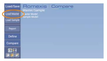
**Note:** The master model is used to compare the two models and evaluate the differences in the preparations. The master model is not necessary if you only want to measure the various areas of the sample model.
