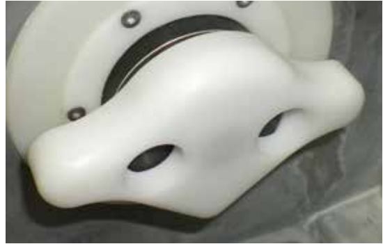
Spindle Cap Tool in locked position - point of the spindle cap pointing down
